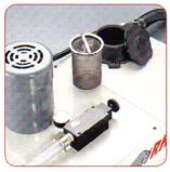
Closed hydraulic tank showing wire screen filter basket for oil return. Adjustable Lexair valve controls oil flow and pressure.
