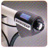
Oil recuperator features a removable stationery plastic support bushing which stabilizes the bar stock thus, eliminating vibration and allowing higher spindle speeds.
