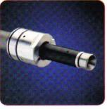
Dynamic bearing-mounted pusher cone maintains contact with bar chamfer allowing much higher spindle speeds.
