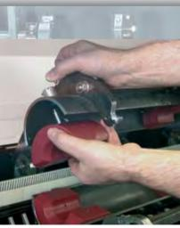
The hydrodynamic and hydrostatic bearing elements are easily accessible, which makes handling them quite simple.
