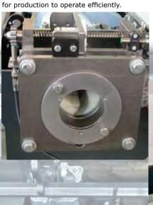
The Hydrobar Sprint 552 and Hydrobar Sprint 565 feature a compact design with all steel machined parts assembled on a heavy duty frame for improved rigidity and performance. Coupled with the heavy duty frame design and depending on production needs, the Hydrobar Sprint 552 and Hydrobar Sprint 565 offer a hydrostatic or hydrodynamic guiding support with or without remnant retract or with an automatic front rest to guarantee optimum RPMs\* without vibration for the entire range of diameters.
