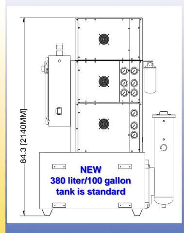
90 liters per minute (24 gpm) <u>Pressure to 80 bar</u> (1200 psi)
