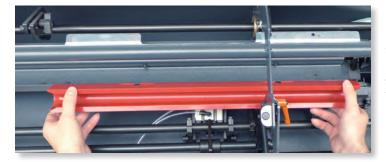
The quick change guiding elements are secured by locating pins, enhancing stability. For complete diameter changeover, the elements can be replaced quickly and easily without tools. The pusher can be simply released by unlocking the quick turn hand levers.
