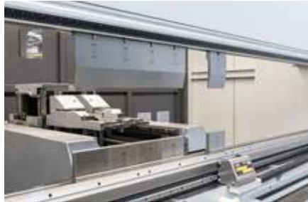
Quick-acting hydraulic clamping installed on the ram.
