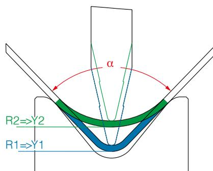
The unique design of the EFL system allows the machine to adapt to material variations such as sheet thickness, strain hardening and grain direction, automatically compensating for any changes.
