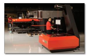
Since FabriVISON is fully integrated with AP100US, inspections can be performed by the machine operator right at the production station. A full scan is completed in seconds while comparing each measurement to CAD specifications. This reduces the time between CAD drawing and first article inspection up to 96%.
