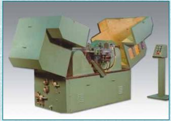
All Fenn Impact Cutoff machines are equipped with a sound-deadening hood.
