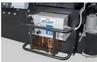
Clean cutting environment is enabled with the mist applicator which sprays cutting fluid to saw blade edges.
