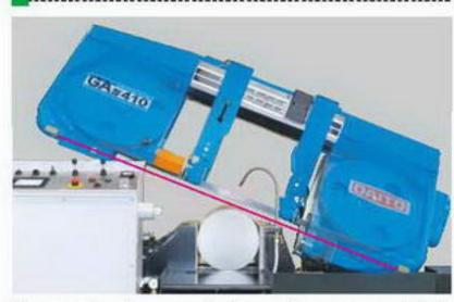
The optical material top detector which checks material top surface is maintenance -free unlike mechanical sensors.
