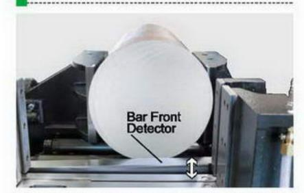
The bar front detector lifts up to detect the front of the material being cut. This makes manual positioning of the first cut unnecessary in automatic cycle.
