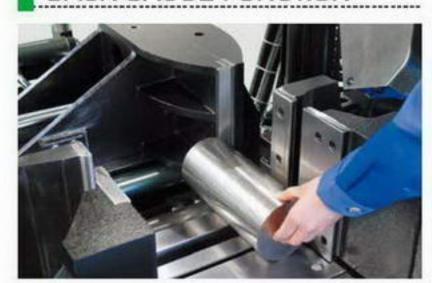
The back gauge function using the index vise is convenient to cut short material in manual mode.
