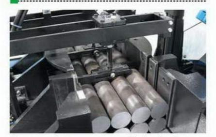
The vertical clamps are installed on both main/ index vises to press down bundled workpiece vertically.
