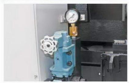
The vise pressure can be adjusted for thin wall material. (Standard feature for USA)
