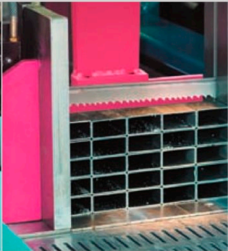
Vertical clamping unit for processing layers and bundles
