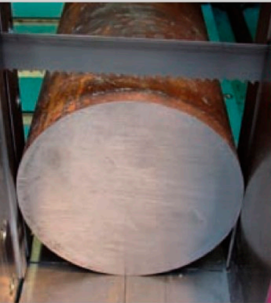
Safe and precise sawing of single bars up to max. 410 mm as well as layers and bundles
