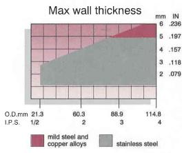
replace welded flange connections, where permitted by the code.
